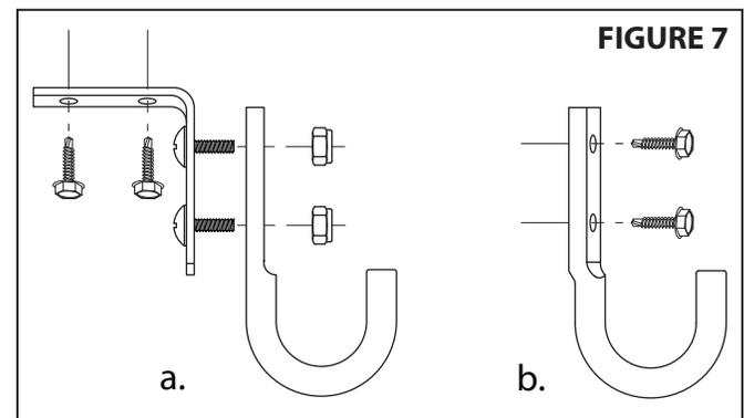
1. Top Mounting (**Figure 7-a**). The hooks may be mounted from the existing headliner screws and hardware, or you may use the enclosed attaching screws. When used with an electric driver these screws are self drilling. For most metals such as aluminum or common steel, they will not require a pilot hole. For some stainless steels however, 1/8” pilot holes will need to be drilled. Attach the right angle mounting bracket to the hooks with the machine screws and lock nuts.
