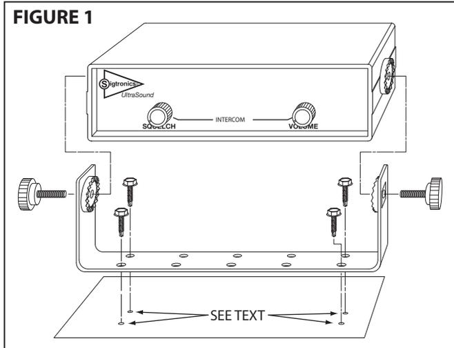
3. The location selected requires a minimum area of 2 5/16 inches high by 7 7/8 inches wide by 4 inches deep. Verify that the intercom unit and cables will not interfere with the normal operation of any vehicle controls or the operation of vehicle compartment doors.
