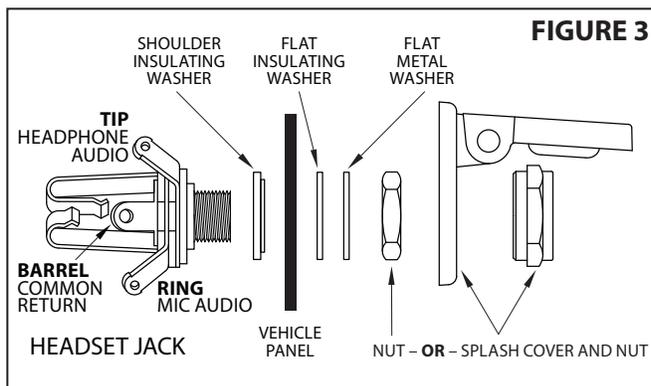
electrical noise getting into intercom system. No need to tighten the jack now. You may have to remove the jack to connect the wires.
