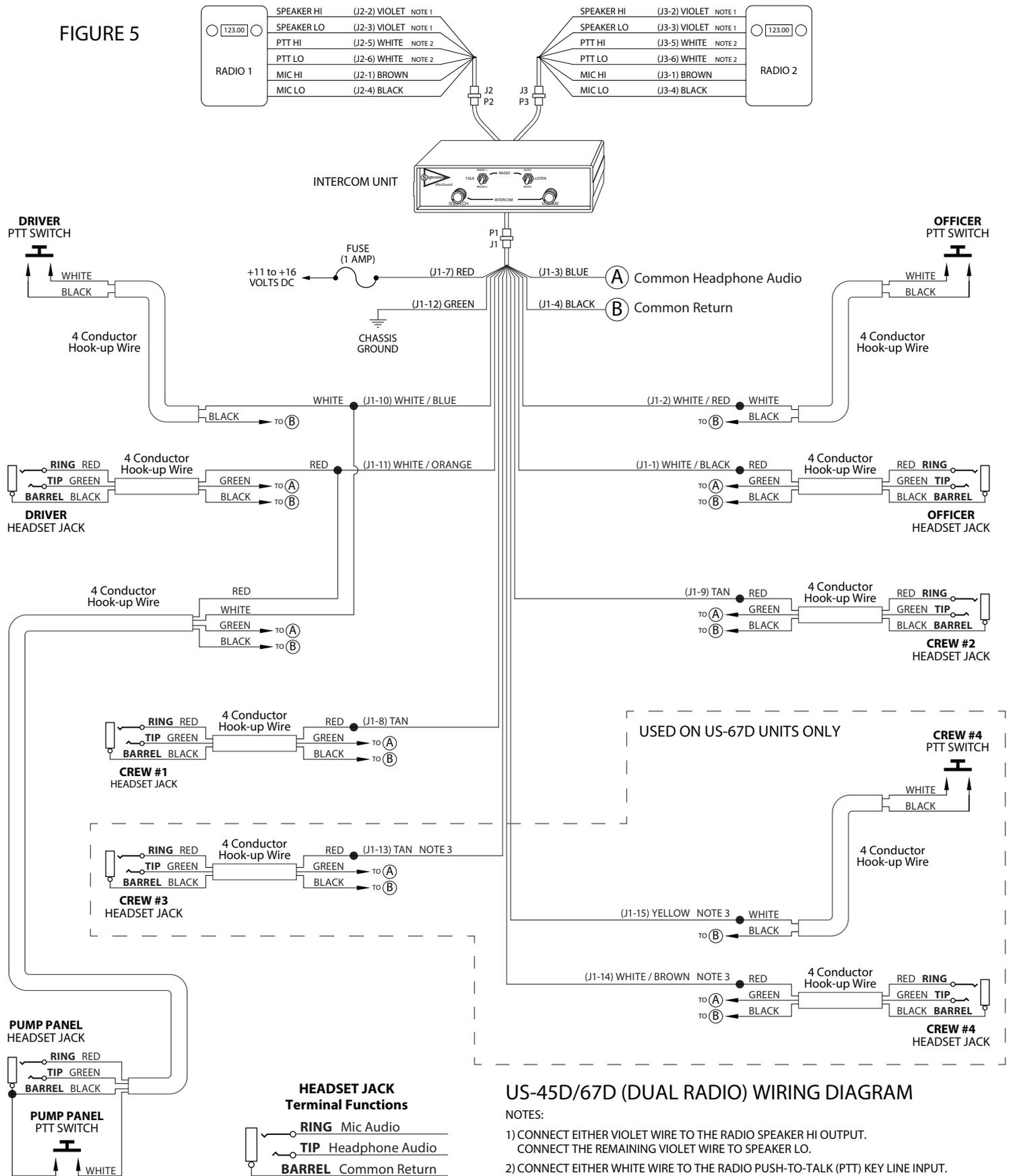
US-45D/67D (DUAL RADIO) WIRING DIAGRAM
