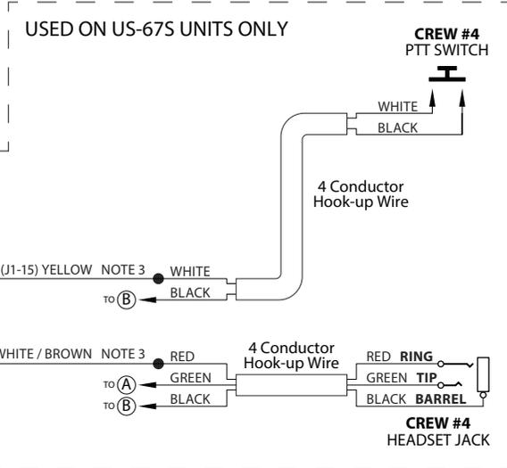
US-45S/67S (SINGLE RADIO) WIRING DIAGRAM
