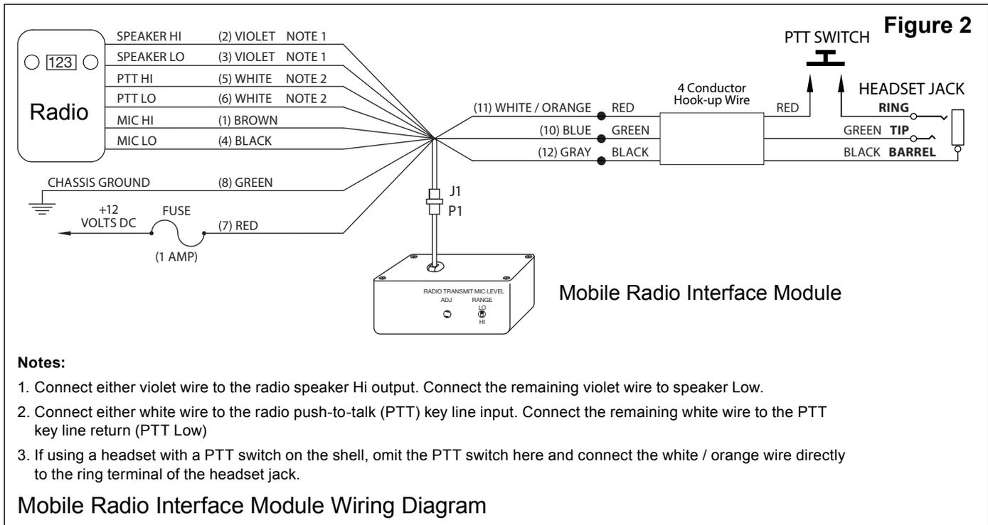
between the Module and radios should be soldered and insulated for reliability. Do not use crimp type splices. Use a good quality electrical tape or heat shrink tubing to cover the soldered connections.
