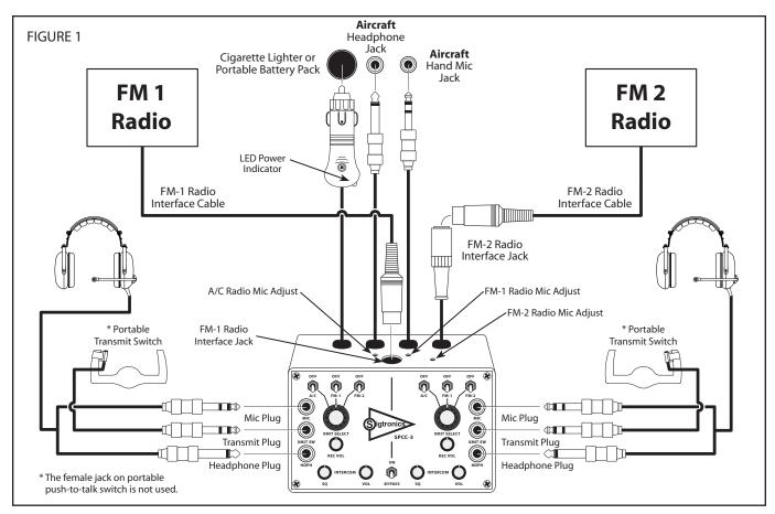
cally adjusts to 12 or 24 volt aircraft. The SPCC can also be powered by an auxiliary battery pack, if desired.
