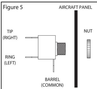
as shown in Figure 4. Identify the jack terminals using Figure 5. Connect the White/Brown, White/Violet, and Black wires to the second jack. Drill a 1/4-inch hole for each jack and mount on the aircraft panel. To use, connect an adapter cable between the music input jack and the output of the portable stereo. Suitable cables are available at your local Stereo or electronics store as well as from Sigtronics.
