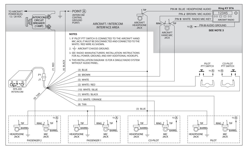
SPA-400 – King KY 97A Radio Installation Wiring Diagram
