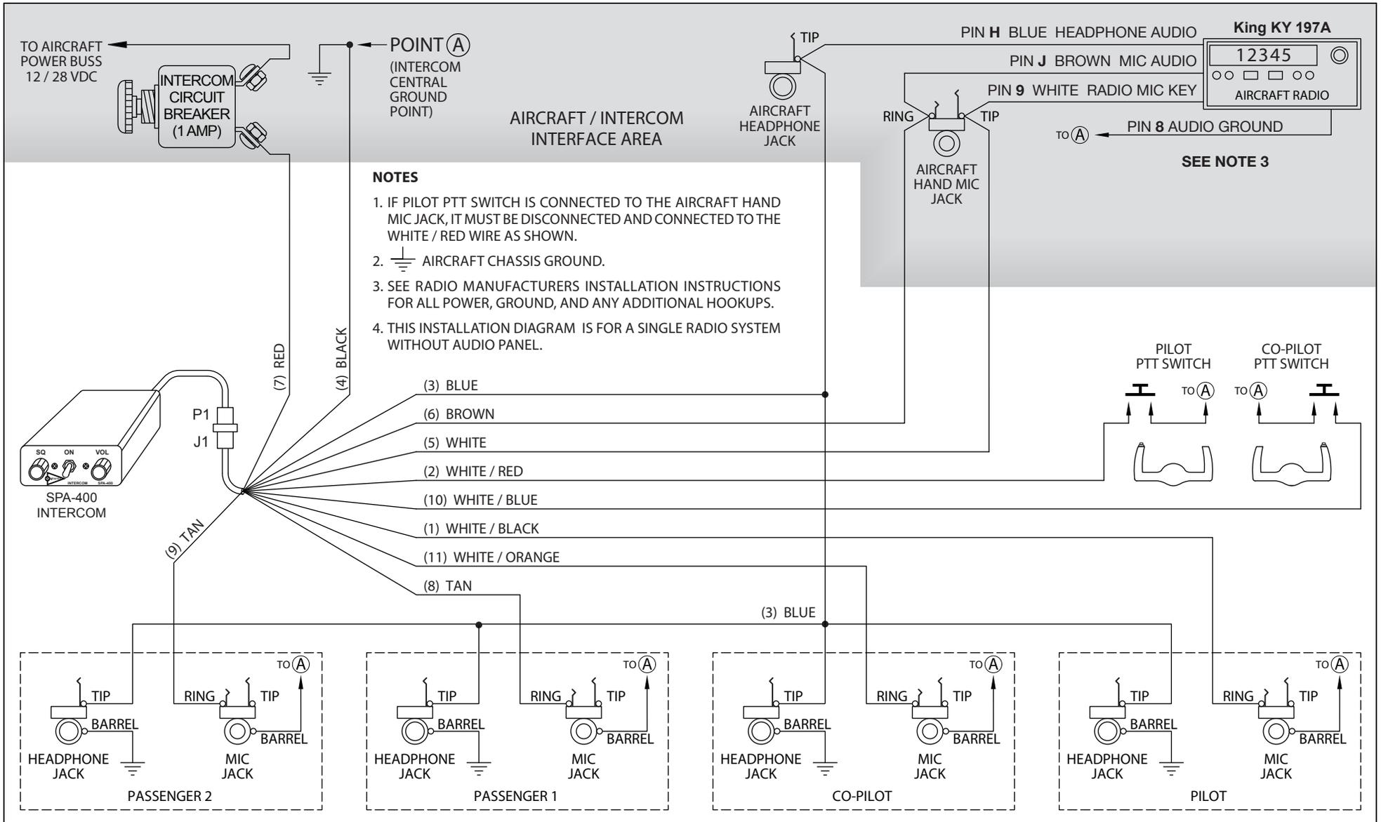
**SPA-400 – King KY 197A Radio Installation Wiring Diagram**
