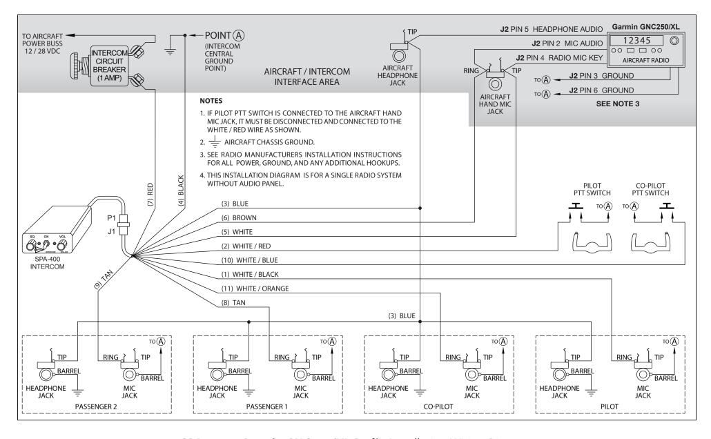
SPA-400 – Garmin GNC250/XL Radio Installation Wiring Diagram
