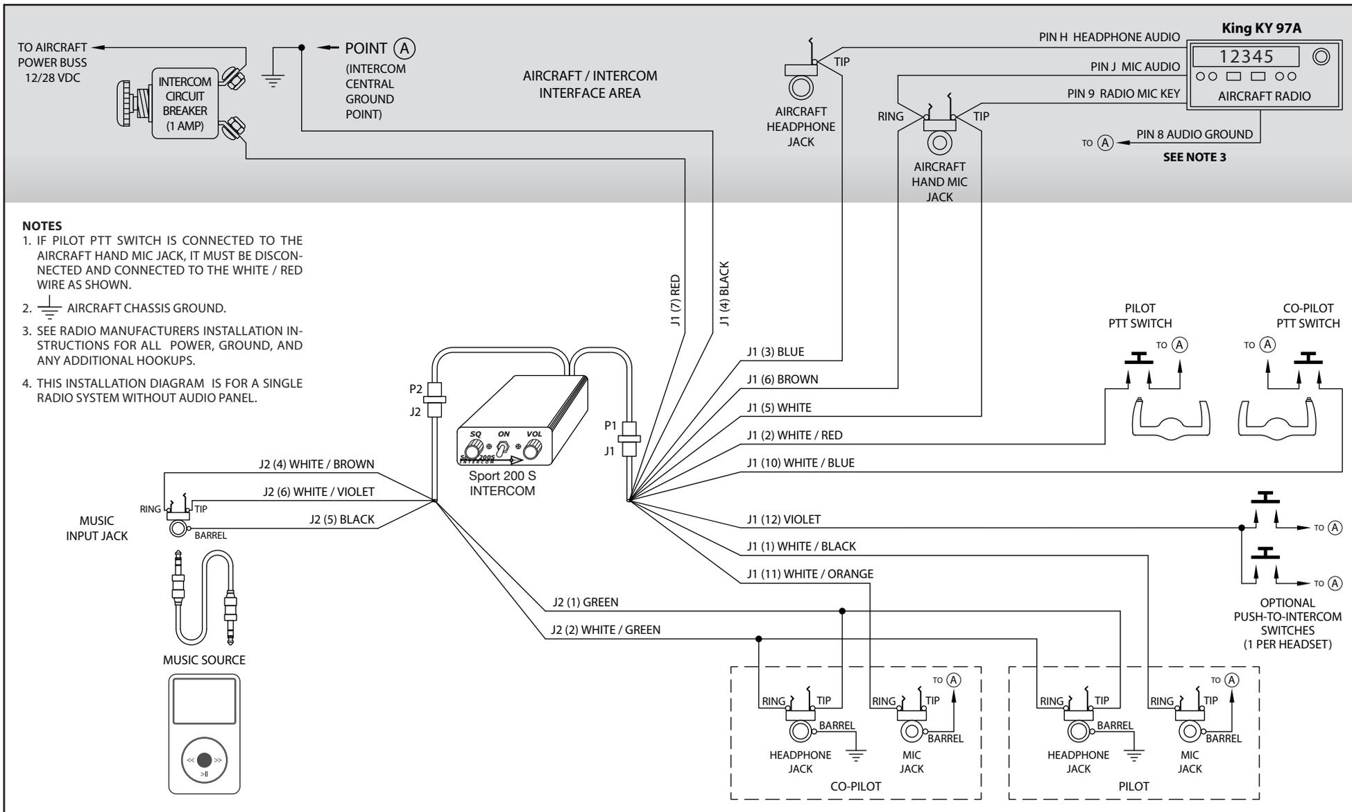
**Sport 200S – King KY 97A Radio Installation Wiring Diagram**
