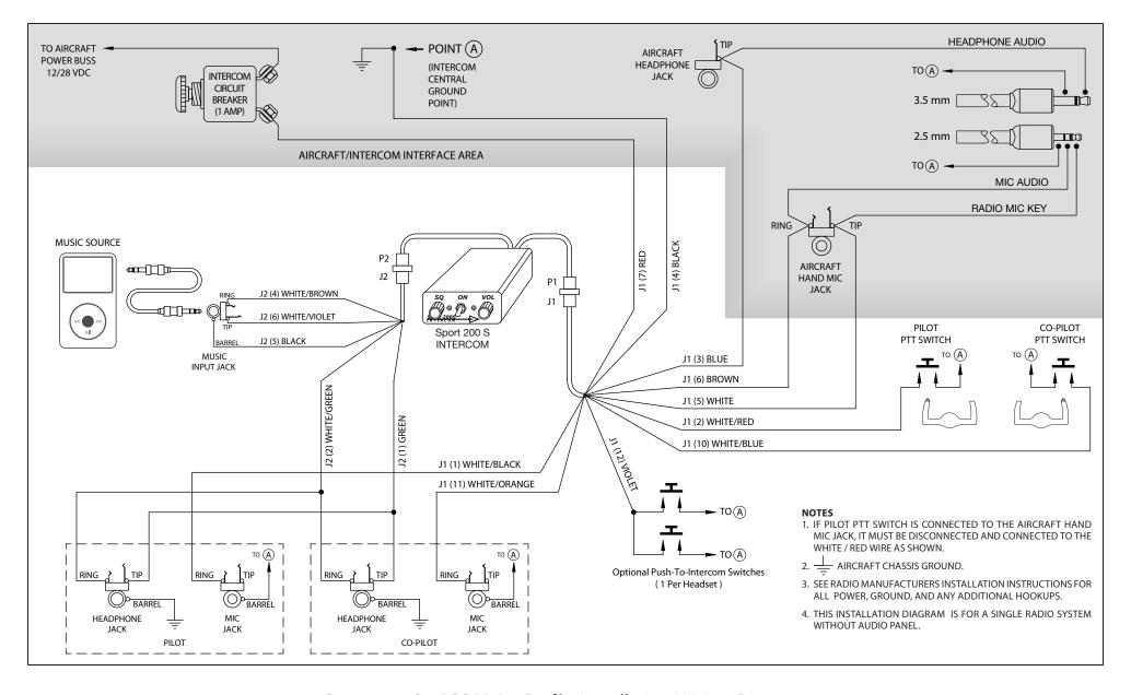
Sport 200S – ICOM A4 Radio Installation Wiring Diagram
