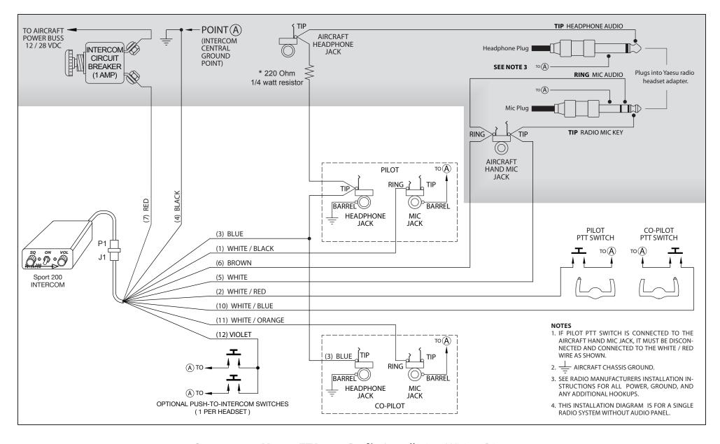
Sport 200 – Yaesu FTA-750 Radio Installation Wiring Diagram
